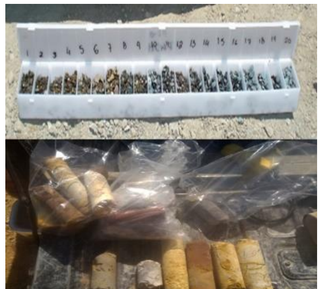
Figure 2. Drill chip samples from RC-drilling and bottom, drill core from the Mathiatis deposit
