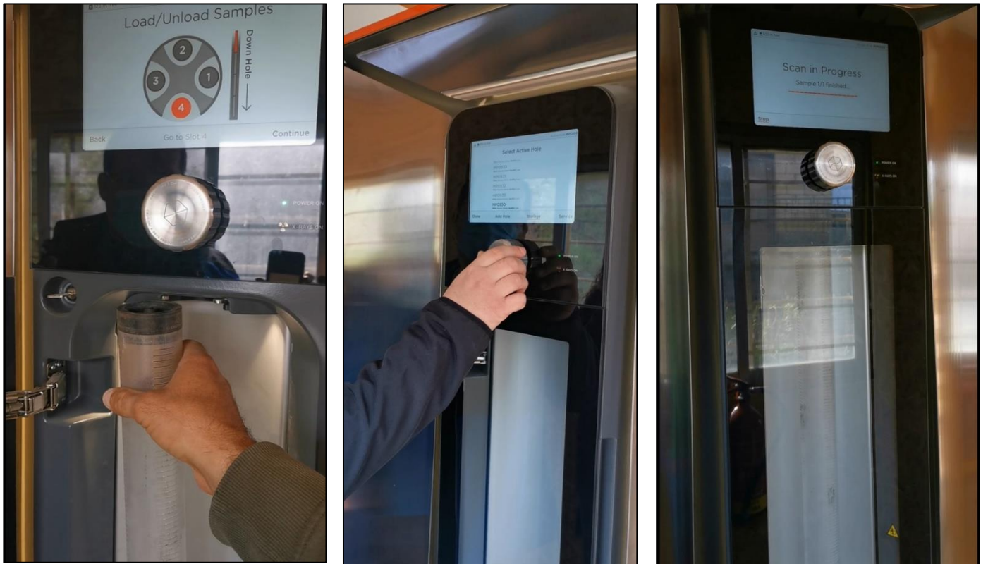
Figure 6. Scanning procedure: inserting the core, setting the depth, scan in progress.
