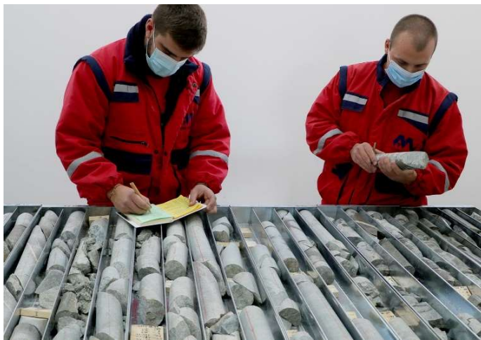
Figure 1. Drill core sampling from Assarel mine
